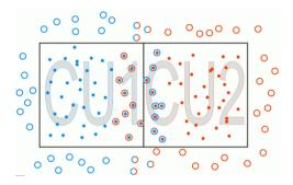
The points used for the computation of the terrain heights in the left CU (no.1) are drawn in blue. The full points are those inside the area of the computing unit, whereas those in the overlap zone are shown as rings. For CU2 (right) the points are drawn in red.
