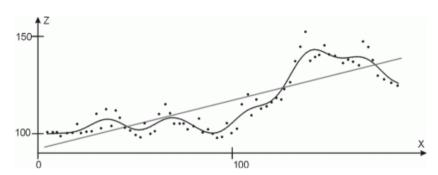
The gray line is the trend which is split off before the computation. In the next figure a histogram of the residuals is shown. For positive values the point lies above the surface.
