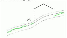
A tolerance band is laid around the coarse surface. The green points are selected. As it can be seen, not only the terrain points are chosen, but also points on the low vegetation.
