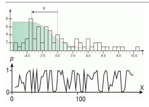
Then repeat the terrain computation under consideration of the weights. Points with high weight will attract the surface while points with low weight will have only little influence on the run of the surface.
