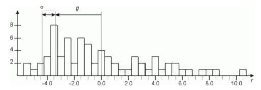
Now, the key idea is the following: Compute weights, individual for each point, depending on the signed distance from the point to the surface. If the distance is positive, the weight shall be low (close to zero), if the distance is negative, the weight shall be high (close to one). The images show the weight function overlayed to the residuals and the weights over the profile ground plan positions.
