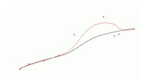
The red surface is obtained with equal weights for all points and the black surface is determined after a few iterations. It is a rough approximation of the terrain surface. In the third step the original points are compared to this coarse DTM, the aim of this step is to **sort out** the original points which are close to the coarse surface. These points provide a finer description of the terrain than on the previous level. It is shown in the following figure.
