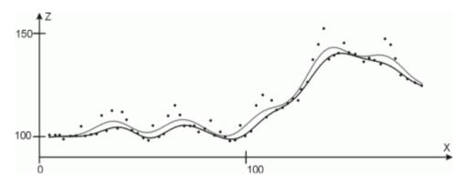
The gray line is the surface from the first iteration where all points had the same weight. The black line is the resulting surface after a few iterations.
