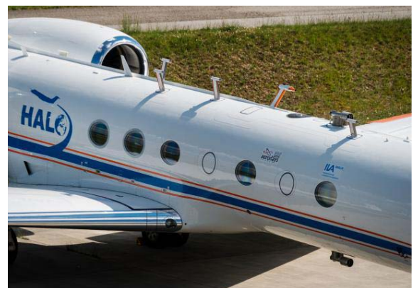
The air inlets on the research aircraft HALO carry air to various measuring instruments inside the aircraft. Credit:DLR(CC-BY3.0)
